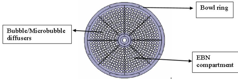
Figure 5. Bubble and microbubble cleaning technique set up
