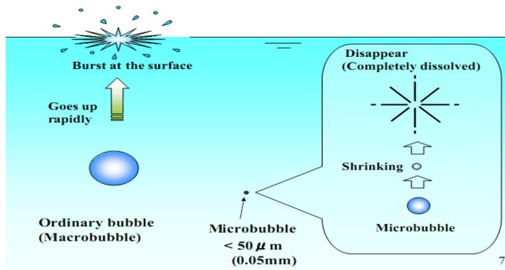
Figure 3. The difference between regular bubbles and microbubbles (Siswanto, 2019)
